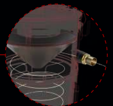
Tangential inlet with cyclone
