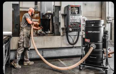
Metal chips cleaning from a CNC machine
