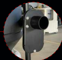
50 mm inlet with sliding damper
